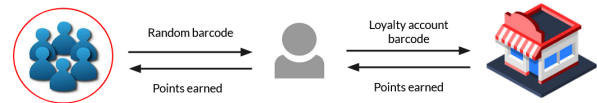
Figure 1: An outline of the solution architecture. From the retailer's perspective, a normal transaction occurs, and the customer provides a loyalty account at checkout time. But because the loyalty account is selected from a third-party anonymity set, the seller is unable to track customer purchasing habits. The customer then relays the number of loyalty points earned, so the third party can keep tally of who owes whom loyalty points.
